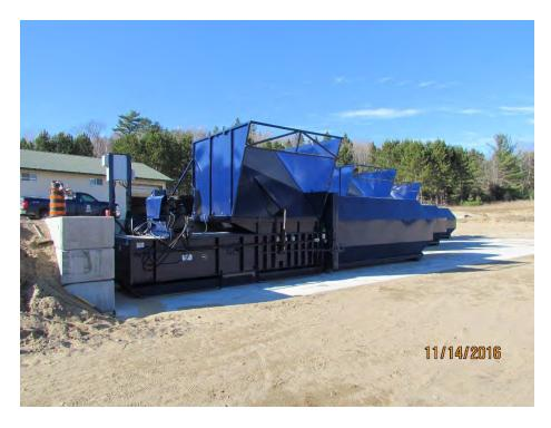
Photo 16 (Nov14-16) Three (3) Blue Box recycling stationary compactors installed on concrete pad.
