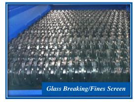
5HP high efficiency variable speed motor per deck, heavy-duty bearings, an automatic oiler and an automatic tensioner, the screen is capable of removing more than 95% of all glass at a throughput of 10 metric tonnes per hour; is low maintenance and has greatly reduced the amount of MRF downtime caused by numerous material jams associated with the original magnetic trommel.
