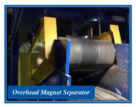
efficiency. The overhead magnet separator recovers greater than 98% of the ferrous containers with less than one (1) percent contamination at 7.5 metric tonnes per hour.
