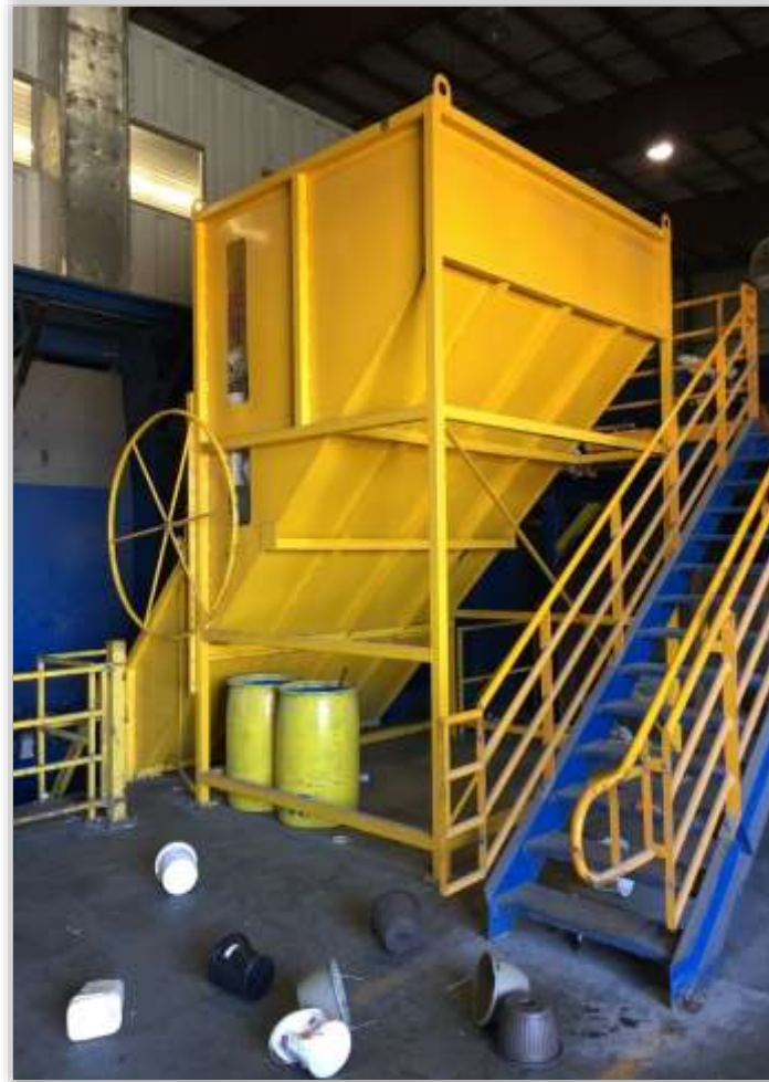
Figure 6: Bunker to capture oversized plastics
