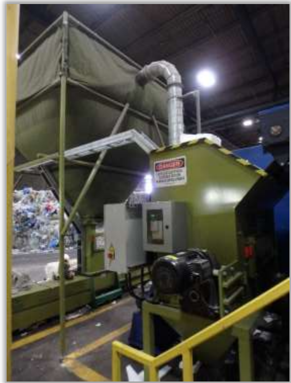
Figure 2 PDS Crusher, Storage Silo and Compactor
