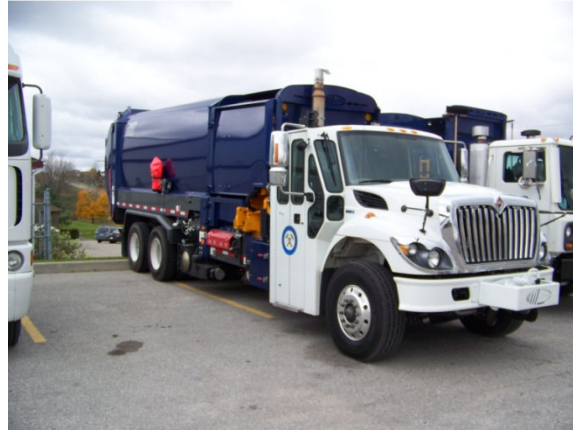
Figure 2: New 35 cubic yard, dual stream automated side loading refuse packer
