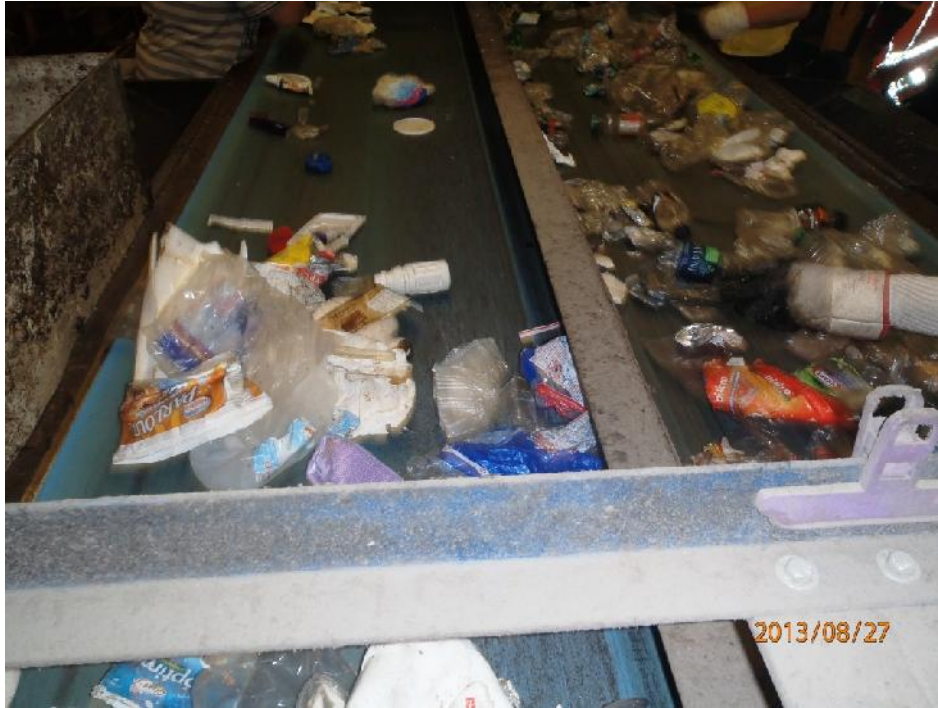
Outbound from sorter: high grade mixed plastics (left) and PET (far right) at QC station
