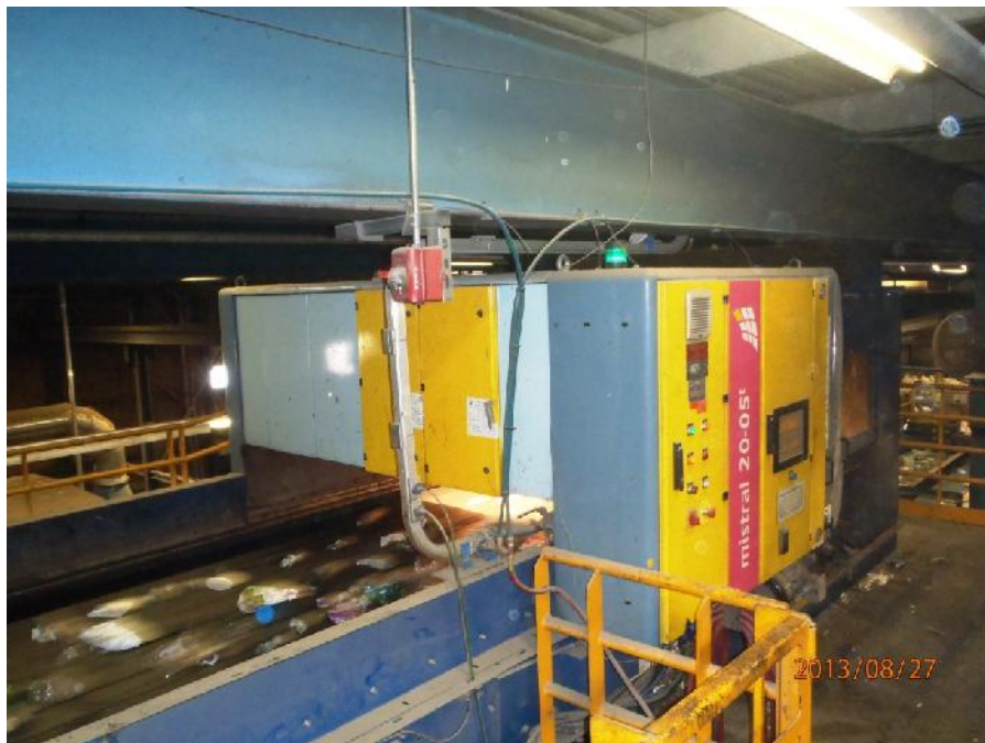
Infeed conveyor for Pellenc Optical Sorter
