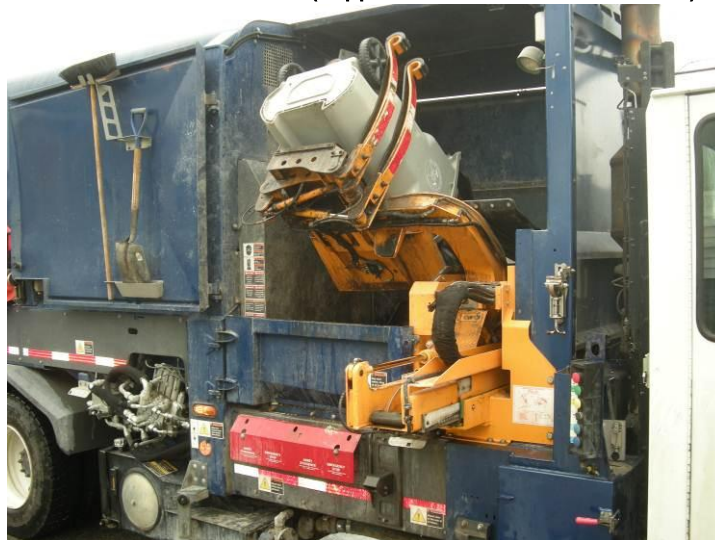
Photo 2 Automated Arm (supported with onboard cameras)
