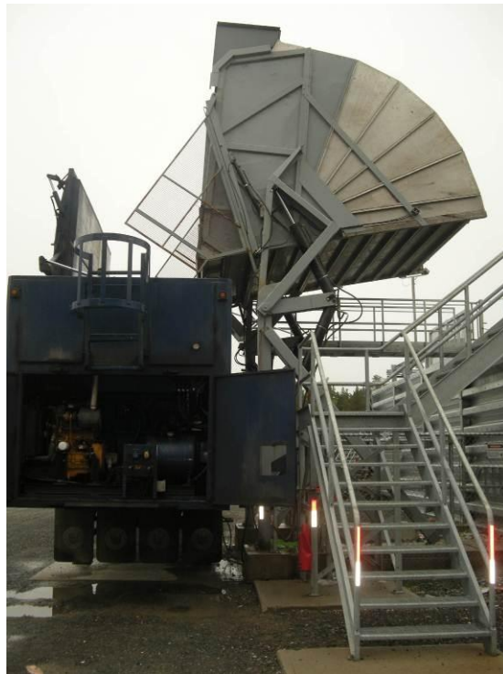
Photo 6 System Supported with Block Heater and Dual Access Walkways
