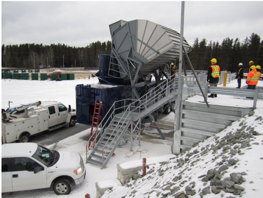
Figure 2: Transtor dumping into Compaction Trailer
