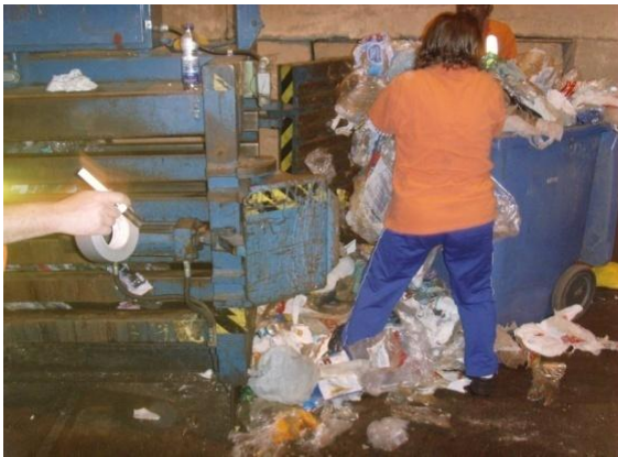
Staff Removing the Plastic Film Bags Inside the Film Baler
