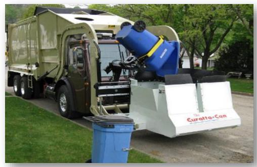
Single or 2-stream trucks; front box can split longitudinally to accommodate different streams
