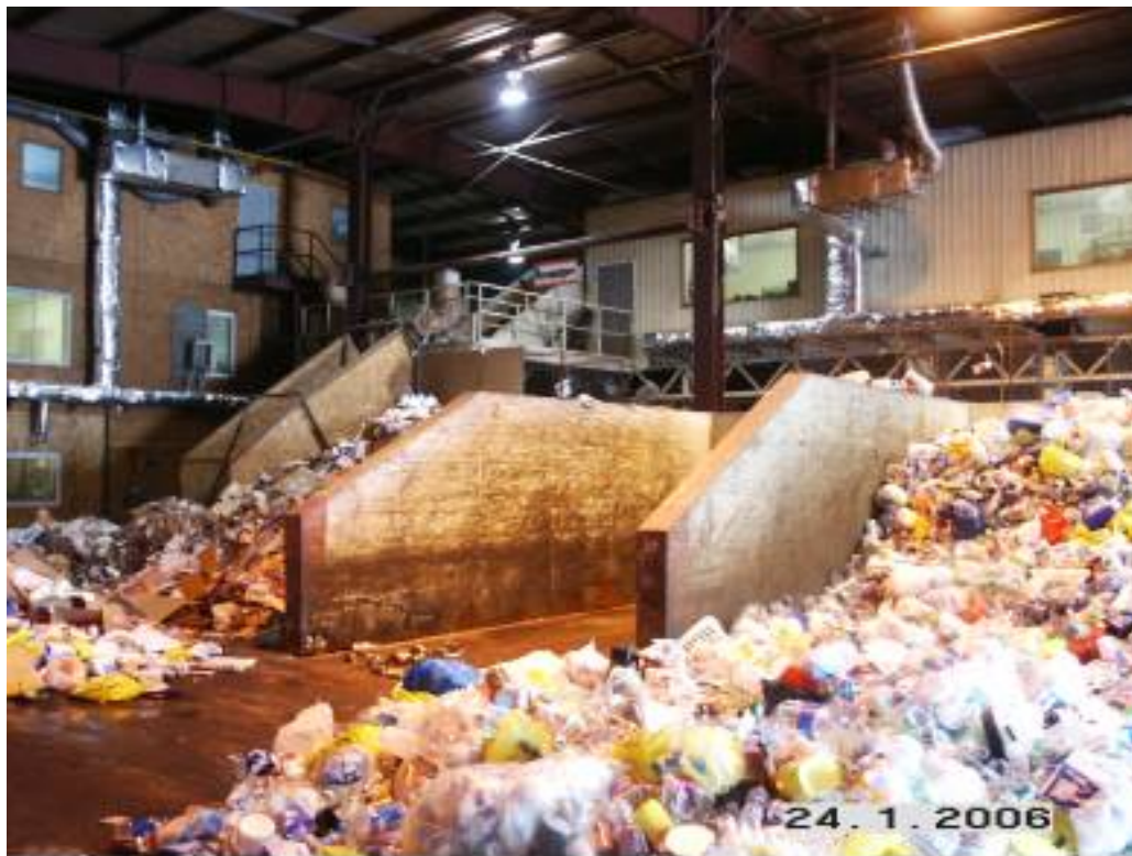
Figure 2-1: RARE Tipping Floor and Sorting Line
